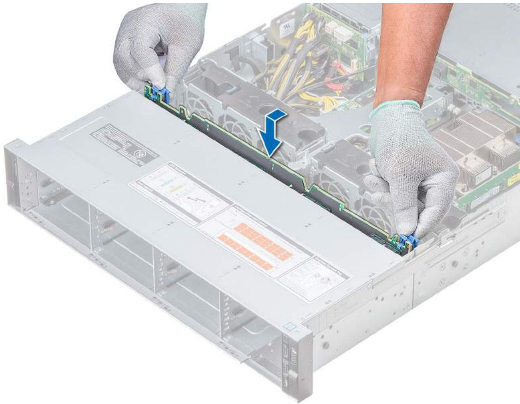
Figure 93. Installing drive backplane
