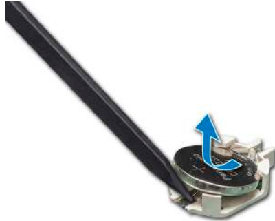
Figure 102. Removing the system battery
