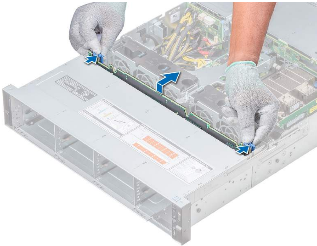
Figure 92. Removing drive backplane
