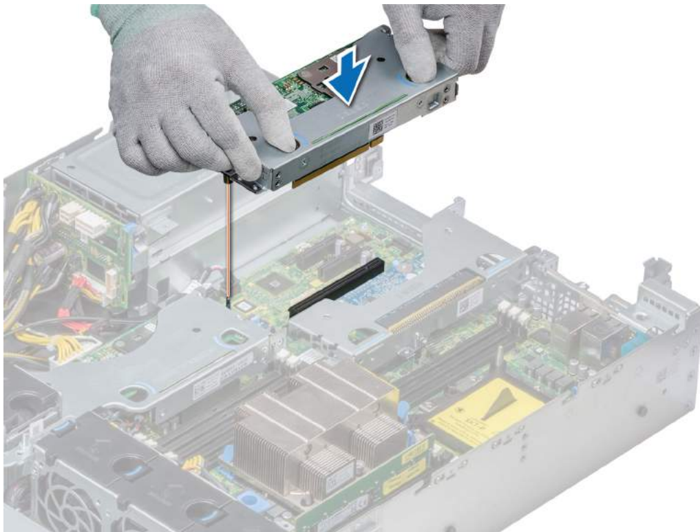
Figure 81. Installing low profile riser left
