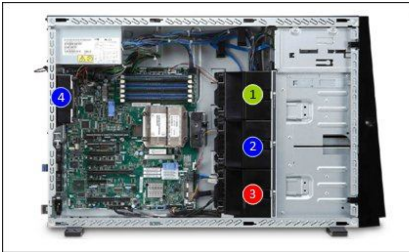
Figure 8. Location of the cooling fans
